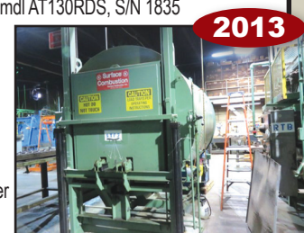
2013 SURFACE COMBUSTION UNI-DRAW Electric Tempering Furnace
